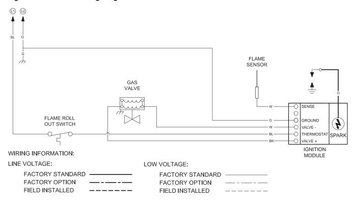
Figure 2.8 • Field Wiring Diagram
