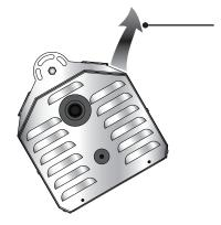
Discharge released from side air channels. Keep area clear of gas piping and electrical wiring.
